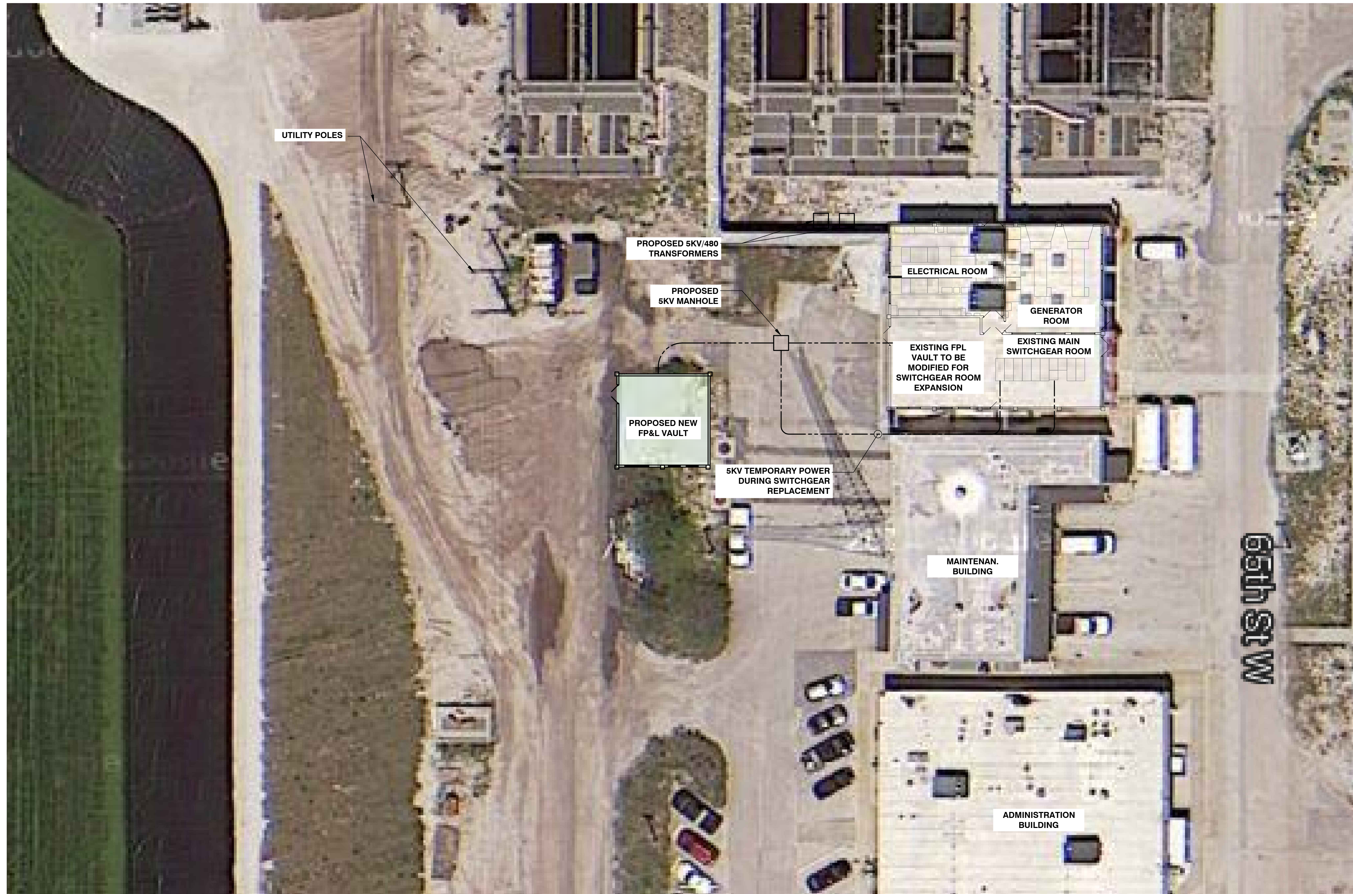
FIGURE No. 7 PROPOSED FP&L VAULT AND SWITCHGEAR LOCATION MANATEE COUNTY - SWWRF ELECTRICAL MASTER PLAN
