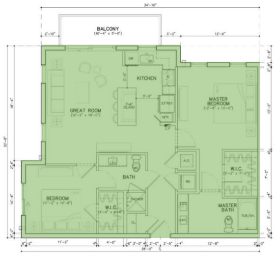
UNIT B3 (280 / 28TH) GROSS A/C AREA = 1074 SQ. FT. (54 DU'S) BALCONY = 82 SQ. FT.
