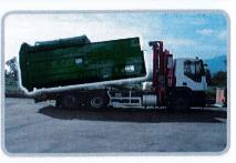
Roll-off Compactor model C.S.N.E. with "Fluctuating blade at Linear Stroke" of new execution, for the collection of compatible and multimaterial (plastic, metal, glass) with the EASY equipment help. Available with hopper 6/7 m³ in volumes ranging from 16 to 20,5 m³.
