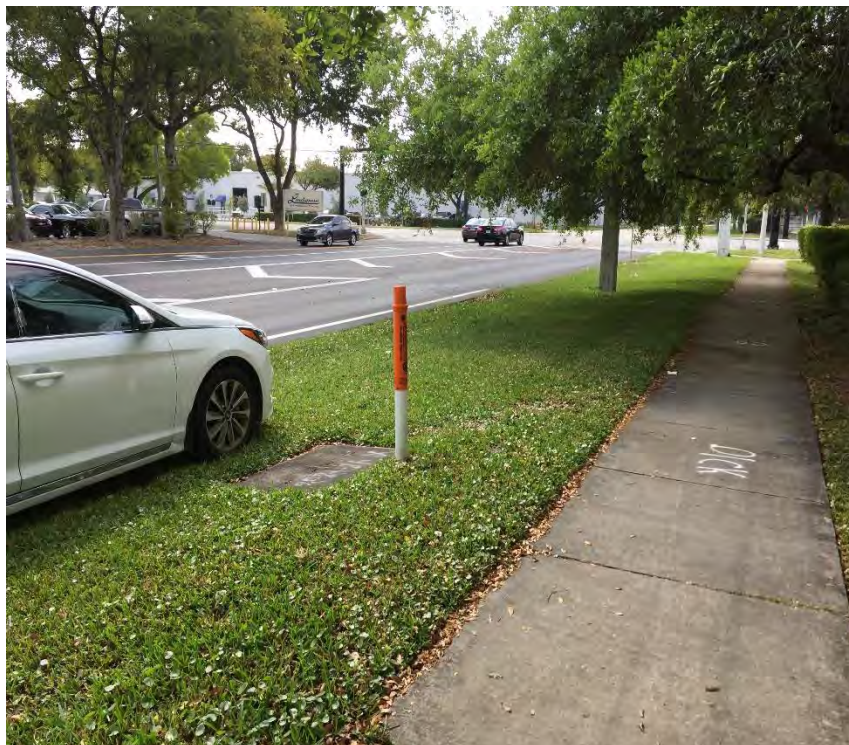
View of a FPL marker indicating that buried fiber-optic lines are located underground (adjacent to east)
