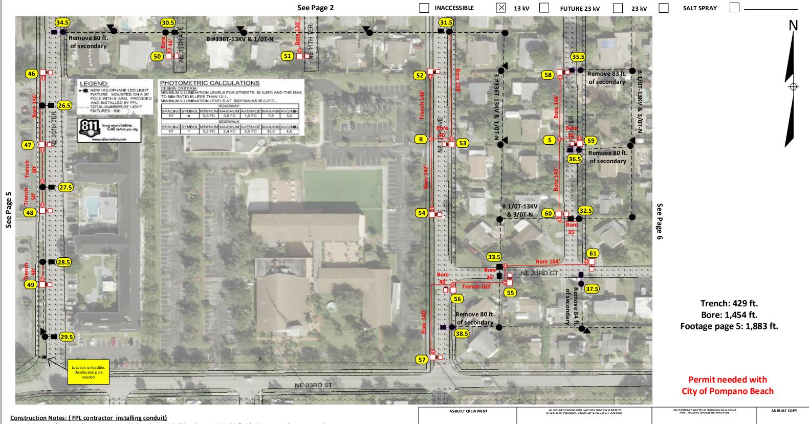
Loc. 46-61: Install 1 Holophane 144W 4K LED Teardrop with 6' bracket on NEW 37 ft. black octagonal concrete pole.
