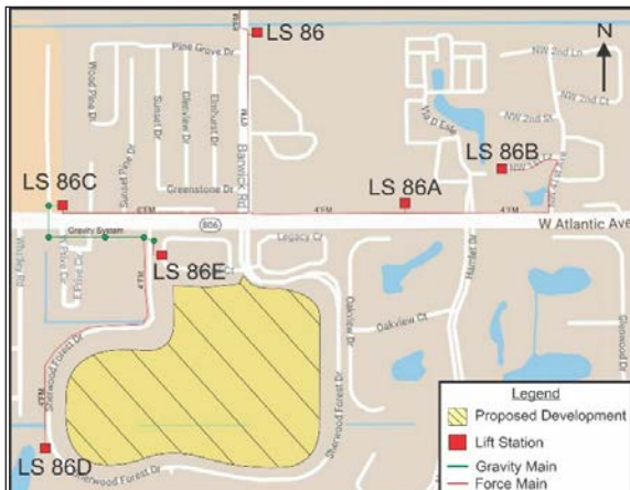
WASTEWATER FORCE MAIN AND LIFT STATIONS
