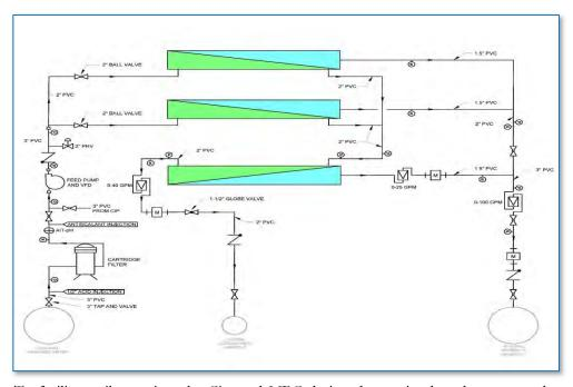
To facilitate pilot testing, the City and MBC designed, permitted, and constructed a pilot unit that utilized full-size (8-inch diameter, 7-element) pressure vessels in a 2:1 array with independent cartridge filters and pre-treatment chemical feed systems. The pilot unit was permitted to withdraw feedwater from the NF process raw water header and discharge permeate and concentrate to the plant's respective headers.
