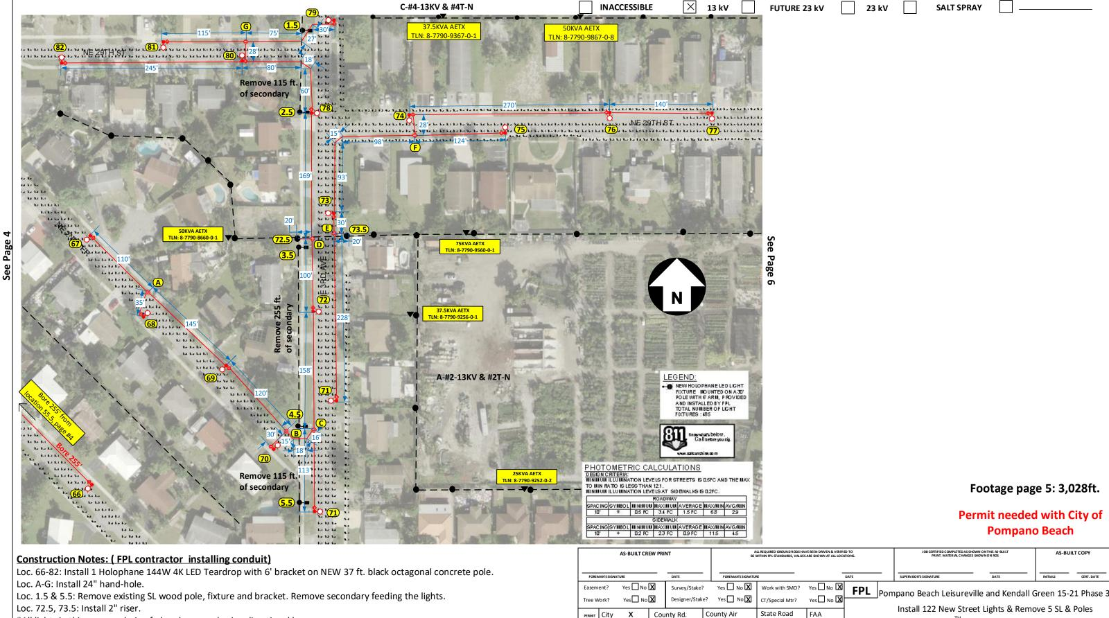
\*All lights in this page are being fed underground using directional bore.
