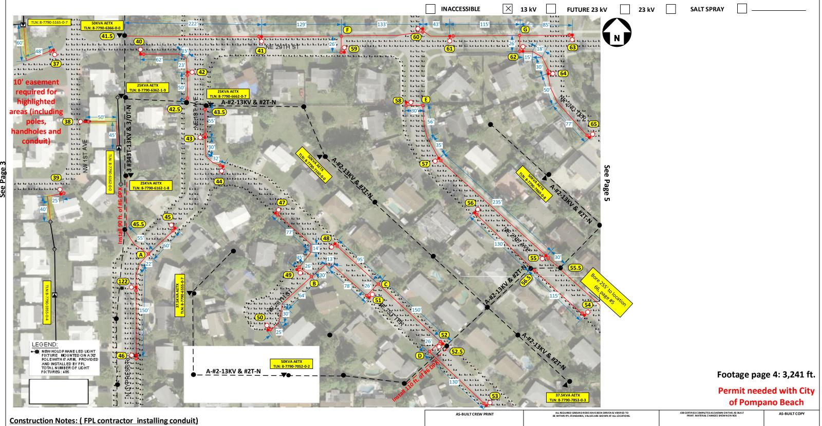
Loc. 37-65: Install 1 Holophane 144W 4K LED Teardrop with 6' bracket on NEW 37 ft. black octagonal concrete pole.
