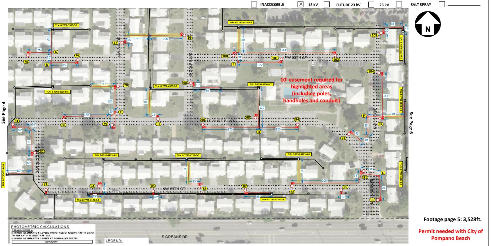
Loc. 75-104: Install 1 Holophane 144W 4K LED Teardrop with 6' bracket on NEW 37 ft. black octagonal concrete pole. Loc. A-G: Install 24" hand-hole.
