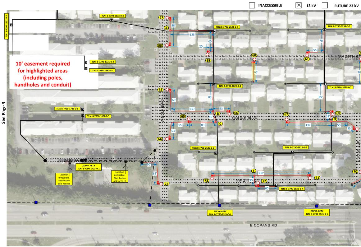
Loc. 57-74: Install 1 Holophane 144W 4K LED Teardrop with 6' bracket on NEW 37 ft. black octagonal concrete pole. Loc. A - E: Install 24" hand-hole.
