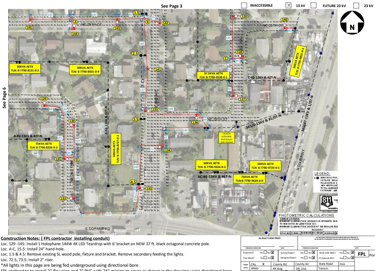
FPL contractor to install 2" flex pipe and 2" PVC with 24" minimum cover as shown in the drawing using directional bore and rapid trench. Cable to be used is #6 DPX UG. FPL contractor installing hand-holes and staking locations of the poles. Poles on this page to be installed in R/W at around 3ft from EOP.
