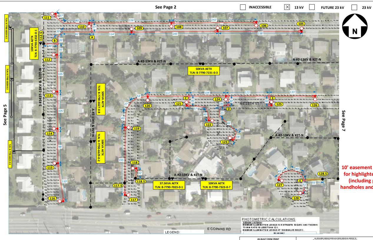
Loc. 105-128: Install 1 Holophane 144W 4K LED Teardrop with 6' bracket on NEW 37 ft. black octagonal concrete pole. Loc. A-E: Install 2" riser and 24" hand-hole.
