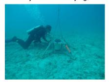
Crandon Marina in Key Biscayne as part of a Sedimentation Study analyzing sand movement into the marina. The data was processed for use in ArcGIS and subsequently used for the numerical modeling of waves and currents, as well as the design of shoreline stabilization structures to ensure a functional solution was developed with minimal impacts to adjacent marine resources.
