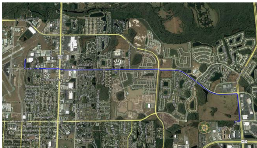
Figure 1.6: LS-116 Force Main, General Alignment and Extents of Inspection
