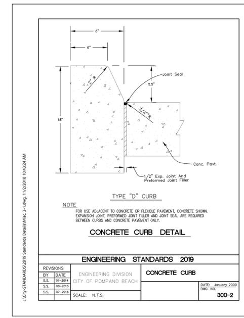
CURB DETAIL PROVIDED FOR REFERENCE ONLY (IF REQUIRED FOR REPAIRS)
