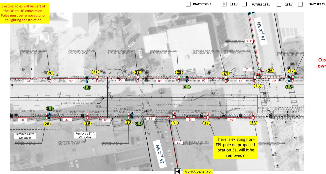
Loc. 20 to 27: Install (1) CREE 144W LED RSW TURTLE FRIENDLY AMB XL (front shield) 4K 5,300 Lumens with 12' Arm Bracket on NEW 30' Standard Arm Mount Concrete Pole Loc. 28 to 33: Install (1) CREE 144W LED RSW TURTLE FRIENDLY AMB XL (back shield) 4K 5,300 Lumens with 12' Arm Bracket on NEW 30' Standard Arm Mount Concrete Pole Loc. 5.5 to 9.5: Remove existing pole, bracket and fixture. Remove OH cable Loc. 20 to 31: Install a 24" HH. Run #1/0 TPX UG cable
