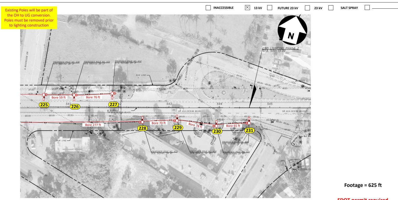
Loc. 225 to 227: Install (1) CREE 144W LED RSW TURTLE FRIENDLY AMB XL (front shield) 4K 5,300 Lumens with 12' Arm Bracket on NEW 30' Standard Arm Mount Concrete Pole
