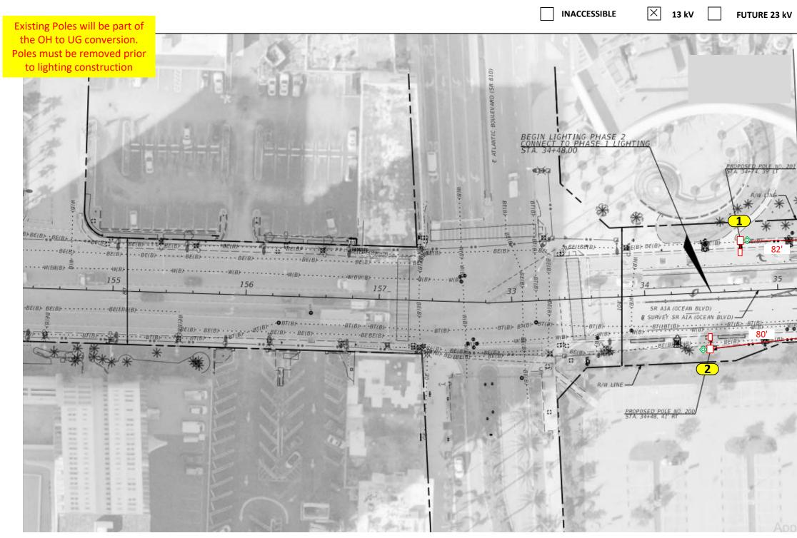
Loc. 1: Install (1) CREE 144W LED RSW TURTLE FRIENDLY AMB XL (front shield) 4K 5,300 Lumens with 12' Arm Bracket on NEW 30' Standard Arm Mount Concrete Pole
