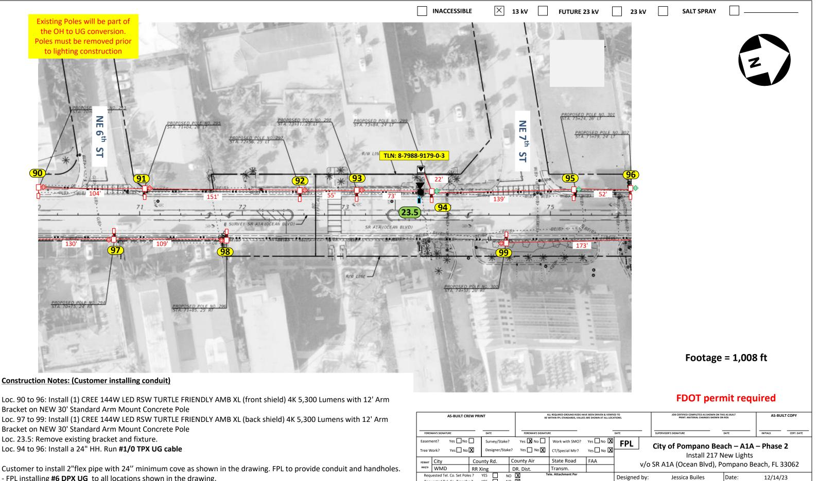
Loc. 90 to 96: Install (1) CREE 144W LED RSW TURTLE FRIENDLY AMB XL (front shield) 4K 5,300 Lumens with 12' Arm Bracket on NEW 30' Standard Arm Mount Concrete Pole
