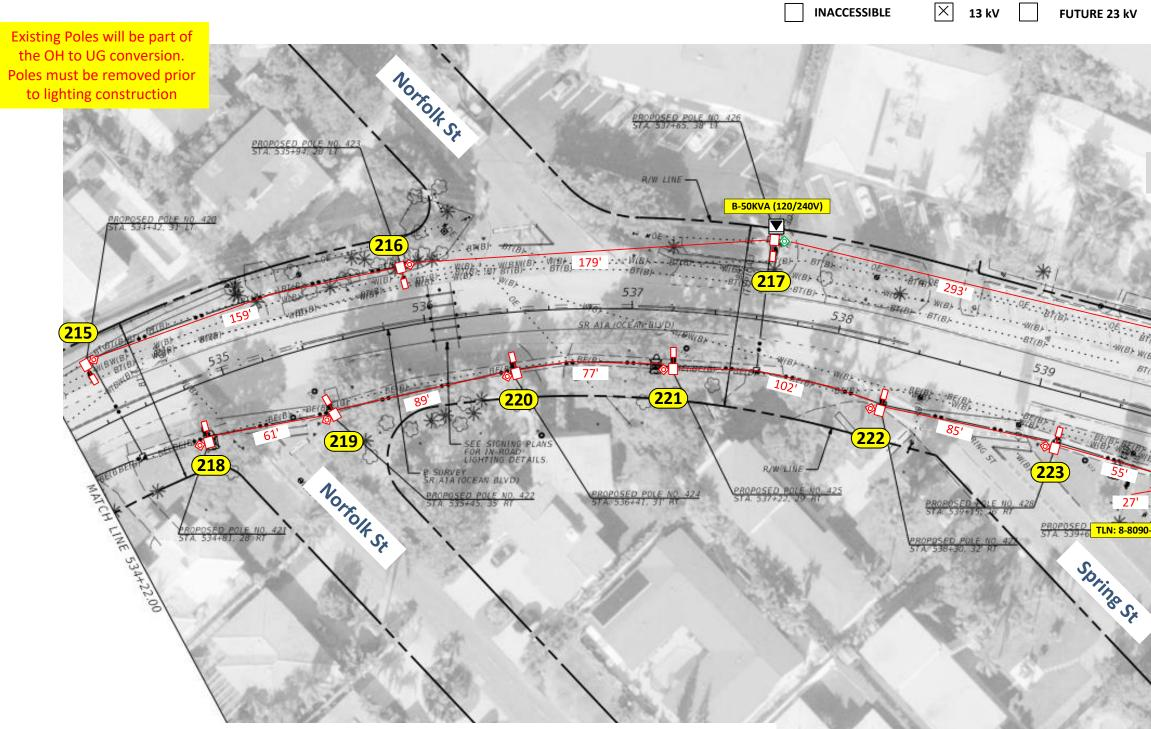
Loc. 215 to 217: Install (1) CREE 144W LED RSW TURTLE FRIENDLY AMB XL (front shield) 4K 5,300 Lumens with 12' Arm Bracket on NEW 30' Standard Arm Mount Concrete Pole Loc. 218 to 224: Install (1) CREE 144W LED RSW TURTLE FRIENDLY AMB XL (back shield) 4K 5,300 Lumens with 12' Arm Bracket on NEW 30' Standard Arm Mount Concrete Pole Loc. 217 and 224: Install a 24" HH
