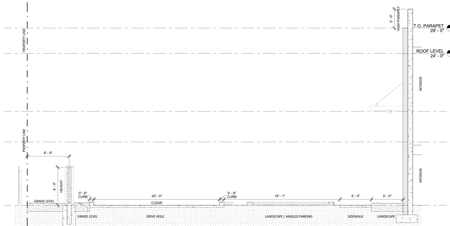
**1 SECTION THROUGH DRIVE AISLE & BUFFER WALL**
