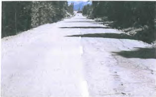
Reclamite was applied to the left-hand lane; the right-hand lane was not treated. This photo, taken five years later, shows severe distress, requiring patching and maintenance. The Reclamite-treated side (left) shows no distress and requires no maintenance.
