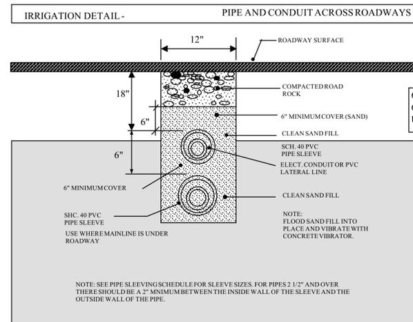
NOTE: SEE PIPE SLEEVING SCHEDULE FOR SLEEVE SIZES. FOR PIPES 2 1/2" AND OVER THERE SHOULD BE A 2" MINIMUM BETWEEN THE INSIDE WALL OF THE SLEEVE AND THE OUTSIDE WALL OF THE PIPE.
