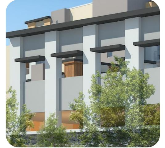
The garage is designed with the same elements as the residential building. Introducing the same aluminum frames (without glass) in the proportion of windows, balcony articulation at the corners of the garage, concrete eyebrows and consistent architectural language as the residential building.
