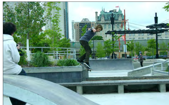
Bio Filtration and Sand Filtration Planters not only provide for creative LID storm water treatment but may serve as integrated skateable elements
