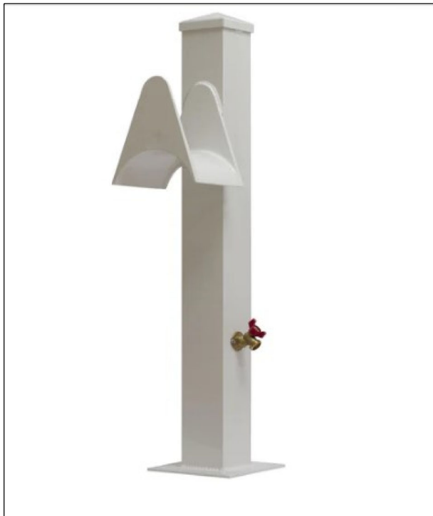
TYPICAL 36" WATER STANCHION 4"x4" ALUMINUM POST W/ 6"x8" ALUMINUM BASE PLATE POWDER COATED WHITE HOSE HOLDER OPTIONAL SINGLE HOSE BIBB SUPPLIED BY INTERNATIONAL DOCK PRODUCTS, DOCK BUILDERS SUPPLY, HAVEN DOCK & MARINE, OR APPROVED EQUAL
