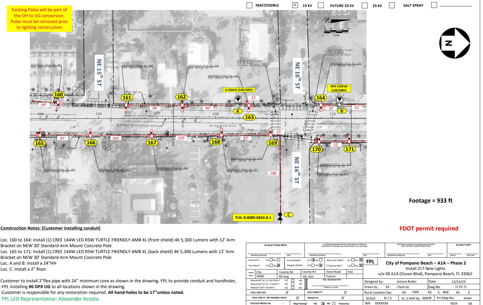
Loc. 160 to 164: Install (1) CREE 144W LED RSW TURTLE FRIENDLY AMB XL (front shield) 4K 5,300 Lumens with 12' Arm Bracket on NEW 30' Standard Arm Mount Concrete Pole Loc. 165 to 171: Install (1) CREE 144W LED RSW TURTLE FRIENDLY AMB XL (back shield) 4K 5,300 Lumens with 12' Arm Bracket on NEW 30' Standard Arm Mount Concrete Pole Loc. A and B: Install a 24"HH Loc. C: Install a 2" Riser
