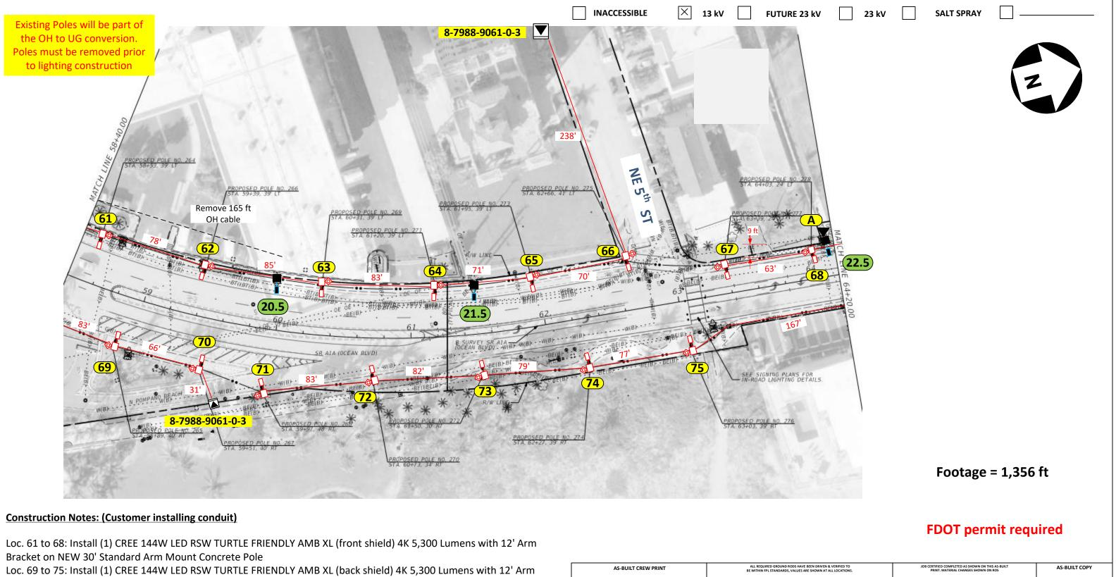
Bracket on NEW 30' Standard Arm Mount Concrete Pole Loc. 20.5: Remove existing pole, bracket and fixture. Remove OH cable Loc. 21.5 and 22.5: Remove existing bracket and fixture.
