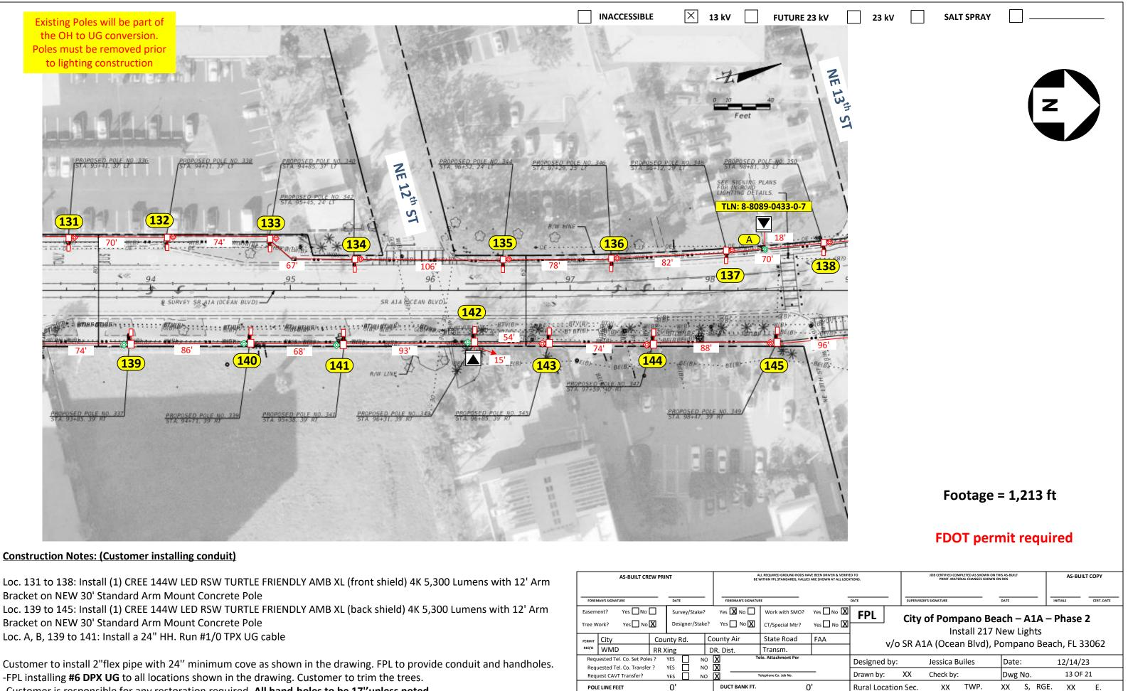
Loc. 131 to 138: Install (1) CREE 144W LED RSW TURTLE FRIENDLY AMB XL (front shield) 4K 5,300 Lumens with 12' Arm Bracket on NEW 30' Standard Arm Mount Concrete Pole
