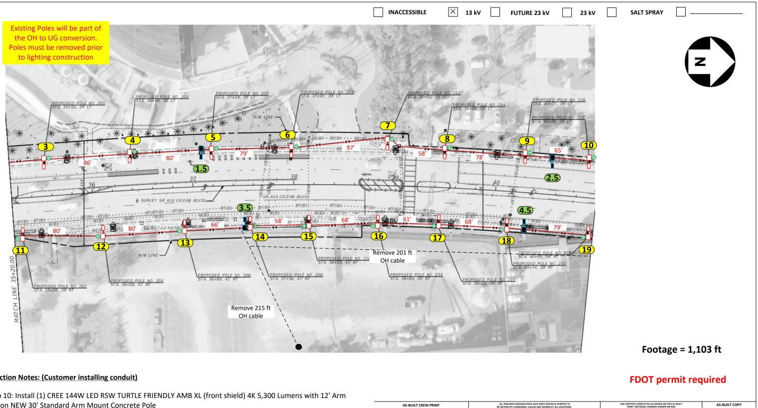
Loc. 3 to 10: Install (1) CREE 144W LED RSW TURTLE FRIENDLY AMB XL (front shield) 4K 5,300 Lumens with 12' Arm Bracket on NEW 30' Standard Arm Mount Concrete Pole Loc. 11 to 19: Install (1) CREE 144W LED RSW TURTLE FRIENDLY AMB XL (back shield) 4K 5,300 Lumens with 12' Arm Bracket on NEW 30' Standard Arm Mount Concrete Pole Loc. 1.5 to 4.5: Remove existing pole, bracket and fixture
