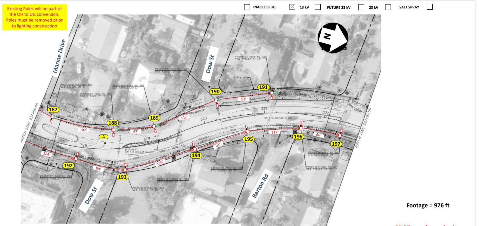
**Construction Notes: (Customer installing conduit)**
