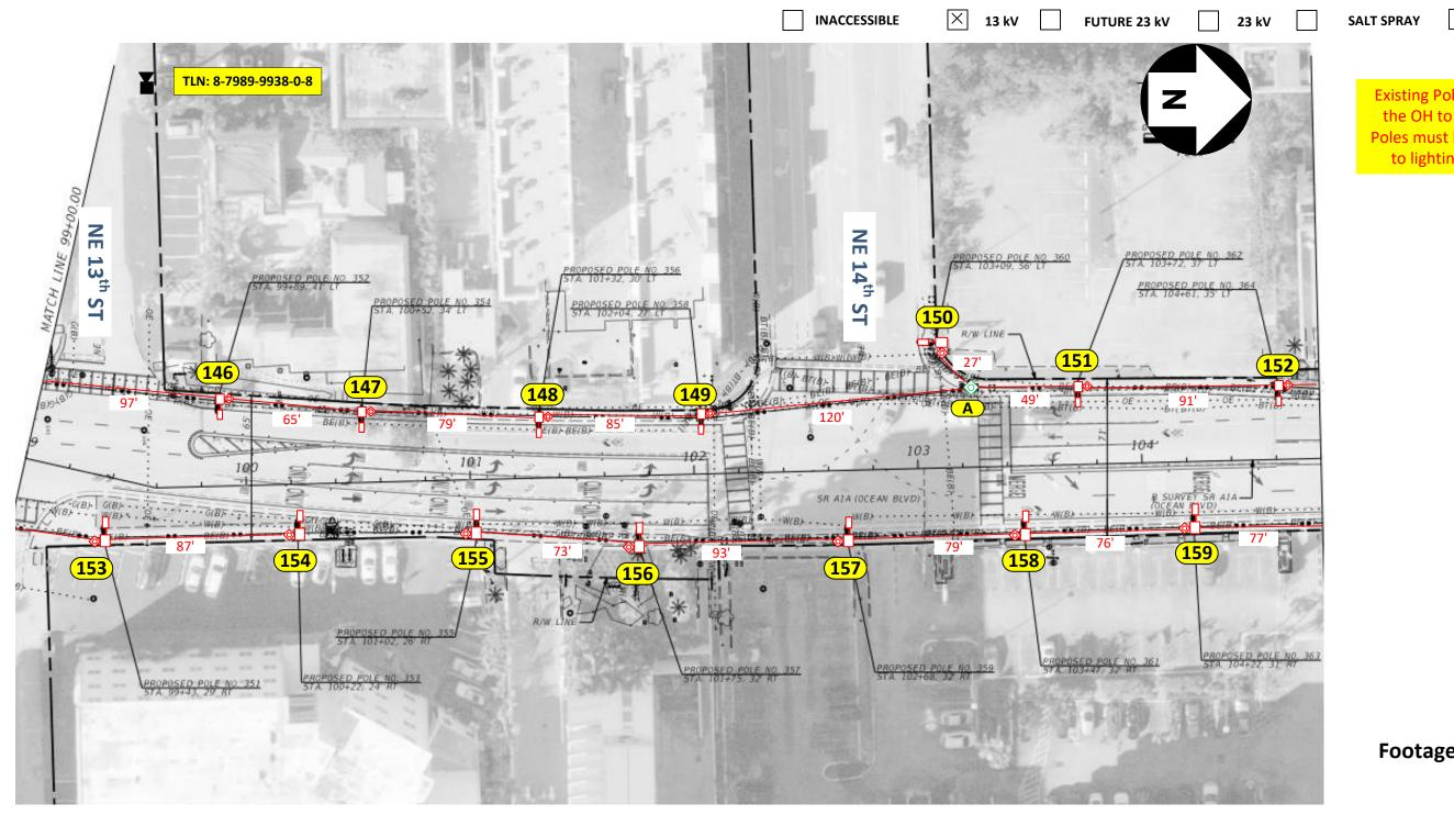
Loc. 146 to 152: Install (1) CREE 144W LED RSW TURTLE FRIENDLY AMB XL (front shield) 4K 5,300 Lumens with 12' Arm Bracket on NEW 30' Standard Arm Mount Concrete Pole Loc. 153 to 159: Install (1) CREE 144W LED RSW TURTLE FRIENDLY AMB XL (back shield) 4K 5,300 Lumens with 12' Arm Bracket on NEW 30' Standard Arm Mount Concrete Pole Loc. A: Install a 24" HH
