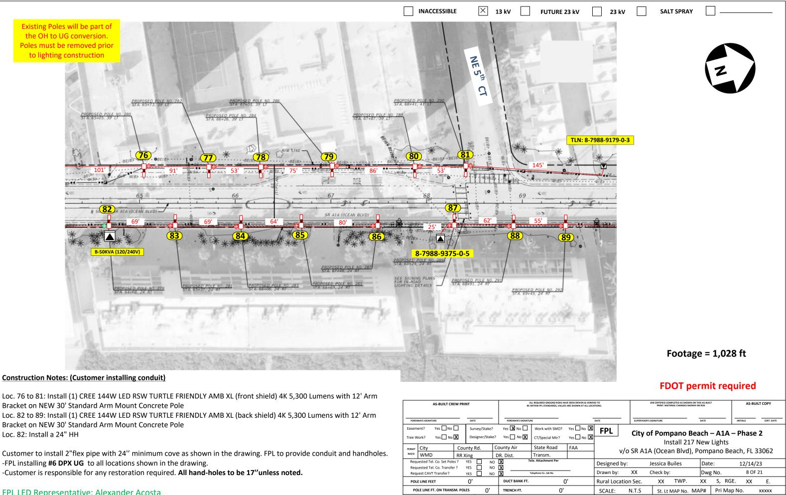
Bracket on NEW 30' Standard Arm Mount Concrete Pole Loc. 82 to 89: Install (1) CREE 144W LED RSW TURTLE FRIENDLY AMB XL (back shield) 4K 5,300 Lumens with 12' Arm Bracket on NEW 30' Standard Arm Mount Concrete Pole
