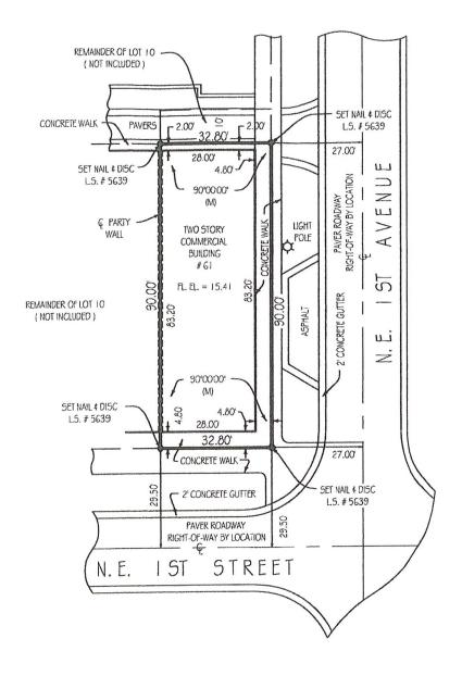
BEARING REFERENCE: NONE. RECORD INFORMATION LACKS ANGULAR DATA. ALL ANGULAR DATA SHOWN BASED UPON FIELD OBSERVATION ONLY.
