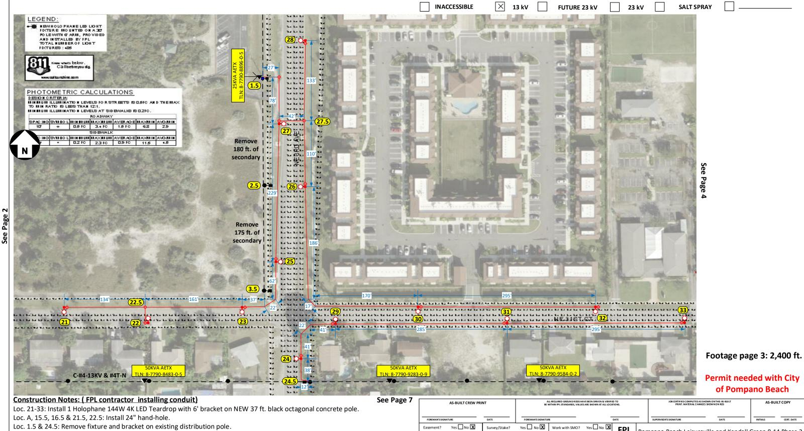
Loc. 3.5 & 4.5: Remove existing SL wood pole, fixture and bracket. Remove secondary feeding the lights.
