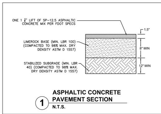
**1 ASPHALTIC CONCRETE PAVEMENT SECTION**
