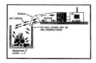
incineration system is a combination of the blower and pit, engineered as a unit to achieve the effect of holding the smoke while feeding air to the fire pit. Since differing site locations contain differing conditions, such as soil composition, water table levels, etc. there are no air curtain incineration systems standards in the industry. In the construction and operation of an efficient air curtain incineration system, special consideration must be given to the following factors:
