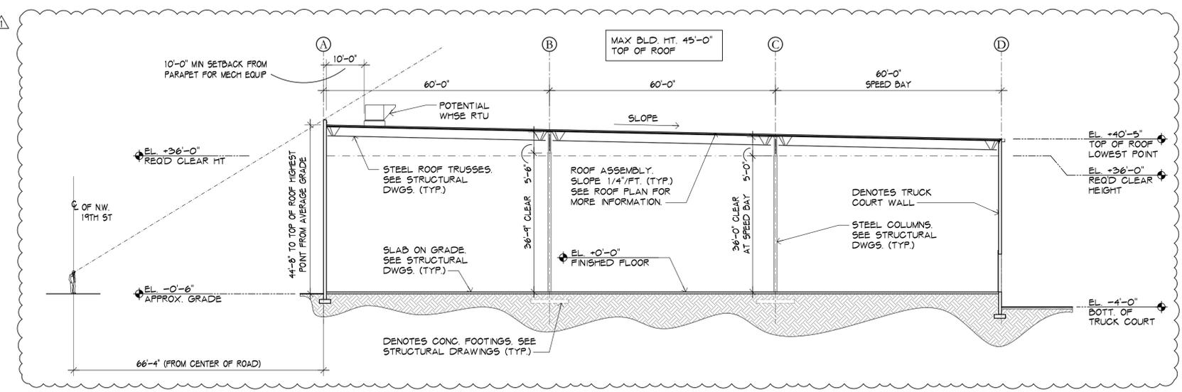
3 EAST SECTION & ROOFTOP SCREENING DIAGRAM AT NW 19TH ST
