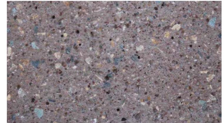
Light sandblast is the least aggressive abrasion type finish. Occasionally referred to as "brush-blast," this finish removes a minimal amount of matrix resulting in a "sandpaper" finish. The amount of aggregate exposed is minimal; due to the natural components used the color and texture will vary. Combination of different levels of sandblasting in conjunction with other casting accents yield dramatic and creative finish options.
