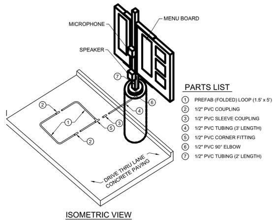
**2 MENU BOARD LOOP DETECTION SYSTEM (ISO. VIEW)**
