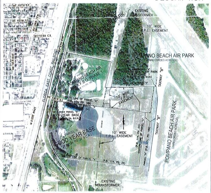
BEARING ARE BASED ON THE SOUTH LINE OF PARCEL "A", POMPANO BEACH AIR PARK F.B.O. PHASE 1 (P.B. 171, PG. 189, B.C.R.) REFERENCE BEARING: N 82'41'26"W THIS IS NOT A BOUNDARY SURVEY
