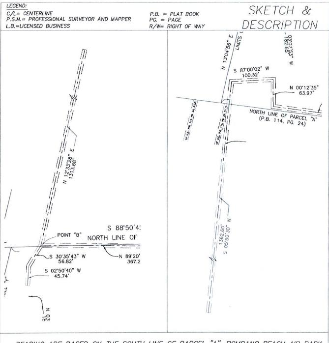
BEARING ARE BASED ON THE SOUTH LINE OF PARCEL "A", POMPANO BEACH AIR PARK F.B.O. PHASE 1 (P.B. 171, PG. 189, B.C.R.) REFERENCE BEARING: N 82'41'26"W
