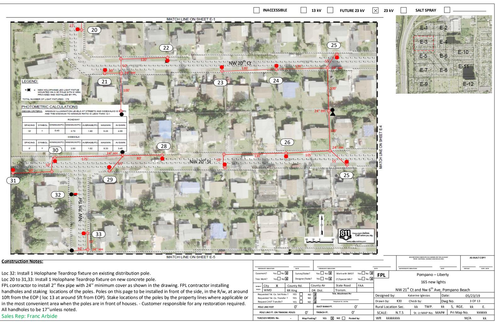
Loc 32: Install 1 Holophane Teardrop fixture on existing distribution pole.
