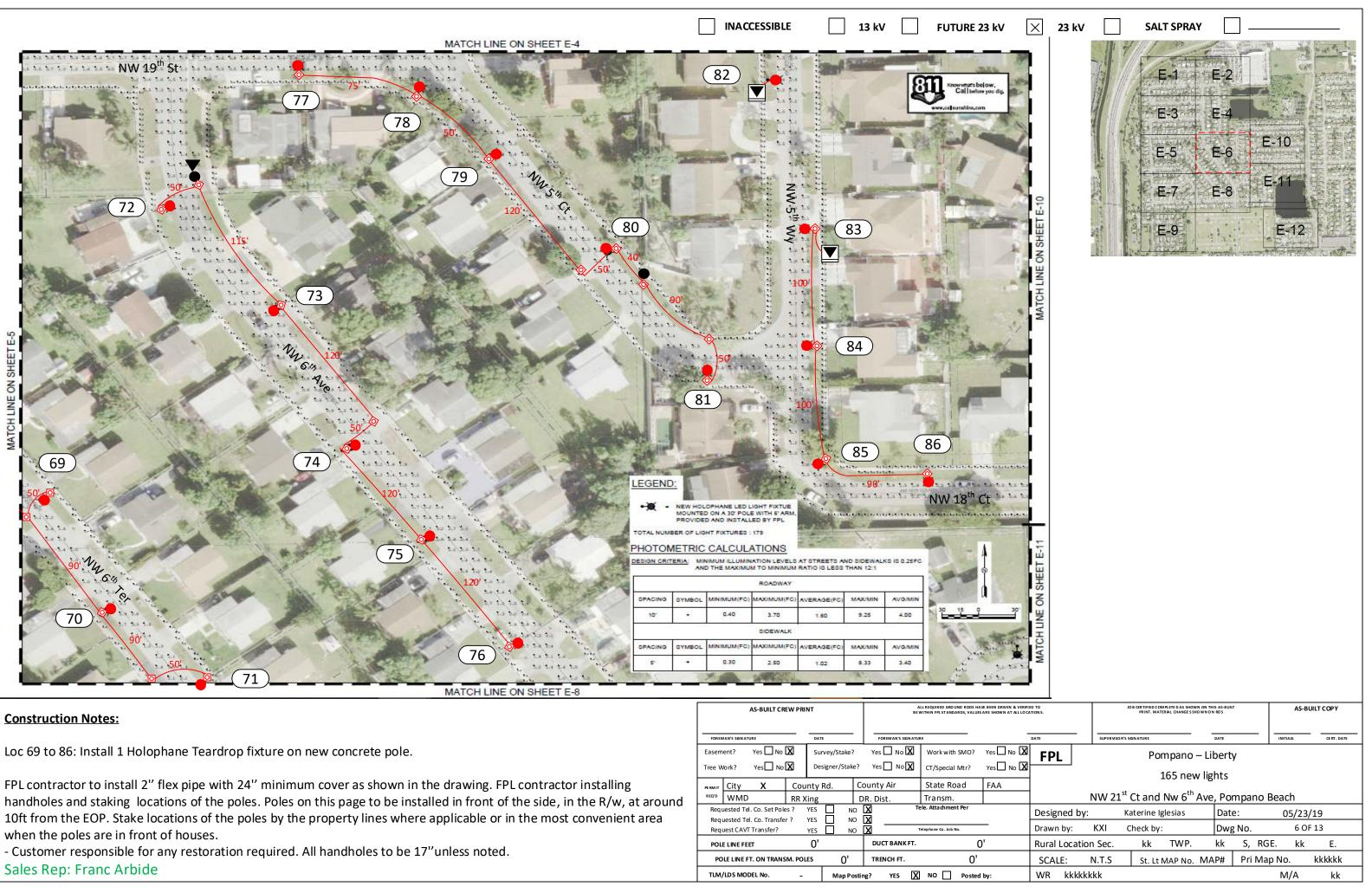
handholes and staking locations of the poles. Poles on this page to be installed in front of the side, in the R/w, at around 10ft from the EOP. Stake locations of the poles by the property lines where applicable or in the most convenient area when the poles are in front of houses.
