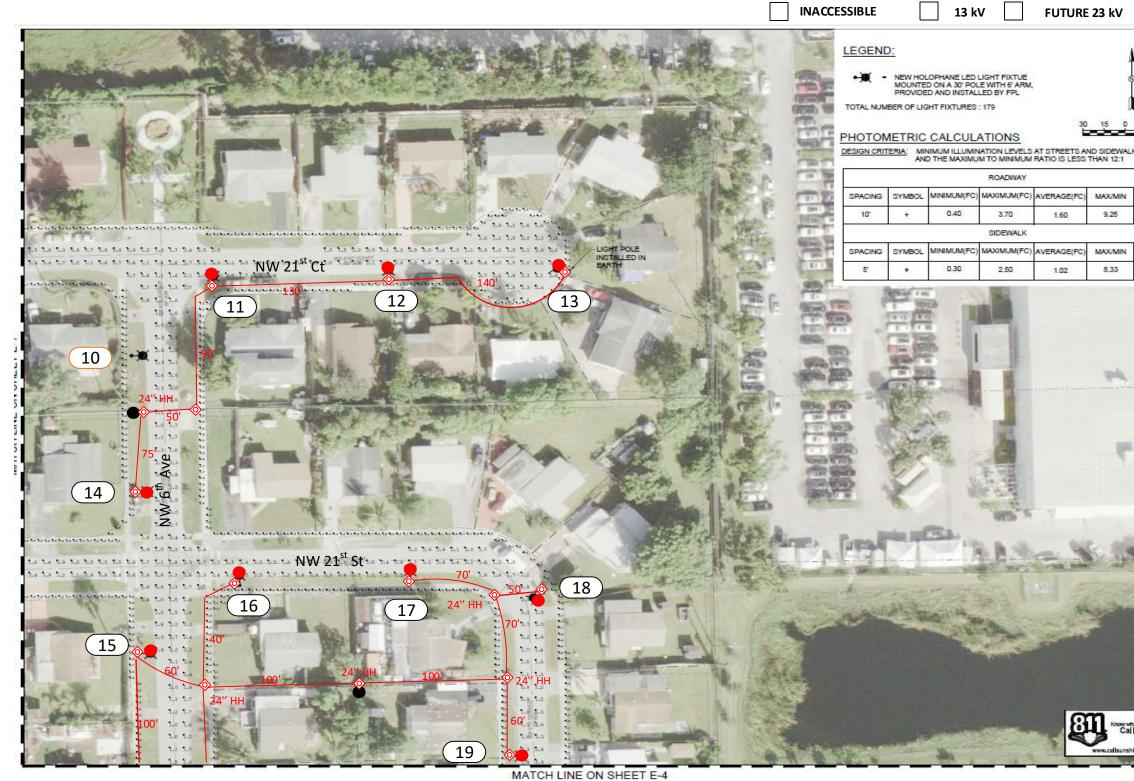
Loc 10: Not feasible, this location is right below distribution lines and it doesn't meet our clearances. Loc 11 to 19: Install 1 Holophane Teardrop fixture on new concrete pole.
