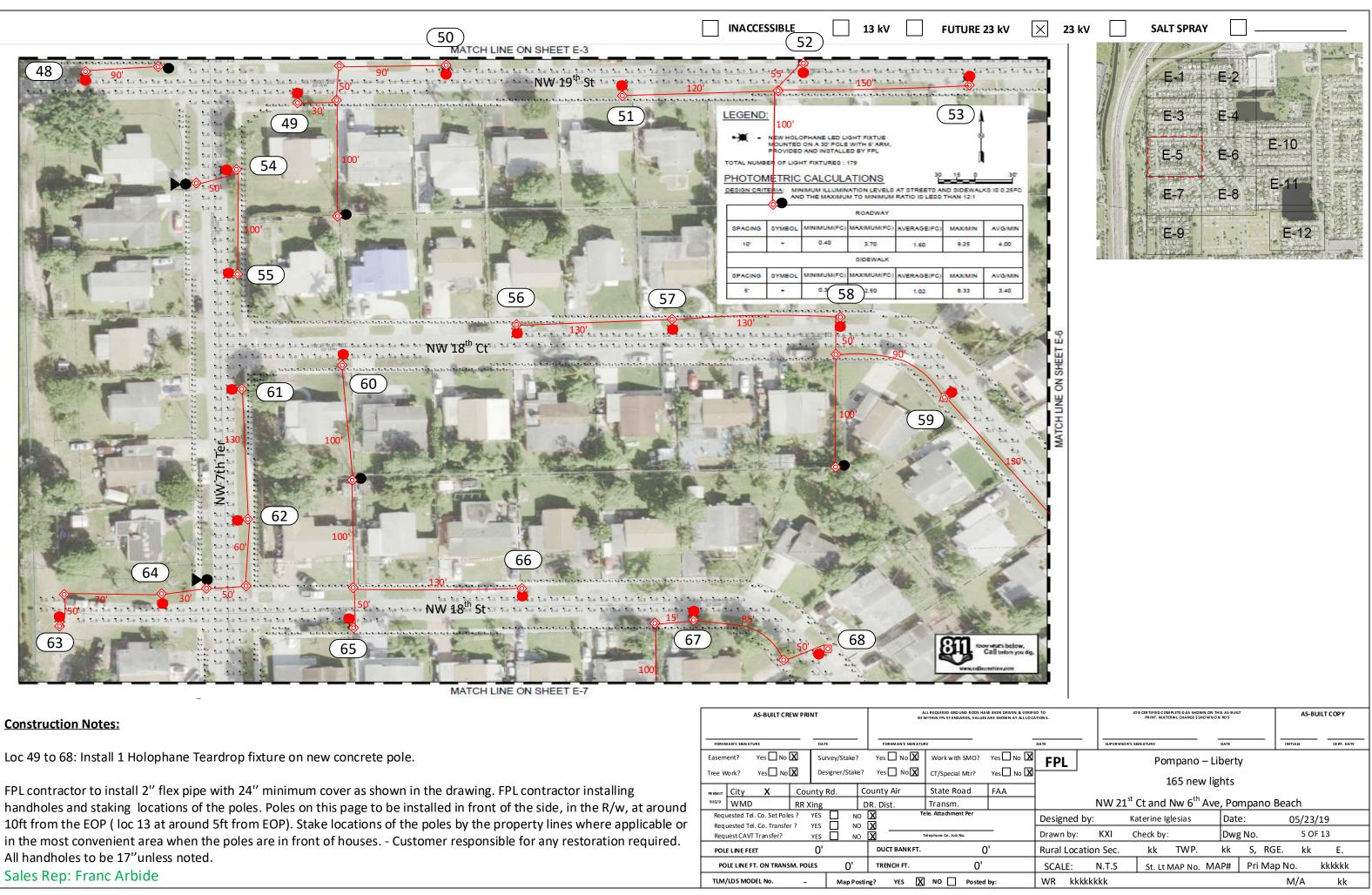
handholes and staking locations of the poles. Poles on this page to be installed in front of the side, in the R/w, at around 10ft from the EOP (loc 13 at around 5ft from EOP). Stake locations of the poles by the property lines where applicable or in the most convenient area when the poles are in front of houses. - Customer responsible for any restoration required. All handholes to be 17" unless noted.
