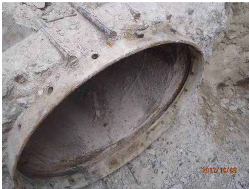
Figure 1: Bell bolt bell exposed with several bell bolts removed
