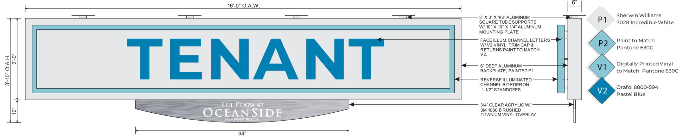
BACKPLATES TO BE ALL ALUMINUM CONSTRUCTION, PAINTED P1. FACES TO HAVE REVERSE ILLUMINATED CHANNEL B ORDER, PAINTED P2 W/ V1 VINYL APPLIED SECOND SURFACE ON CLEAR BACK POLYCARBONATE FOR TEAL BLUE ILLUMINATION. LOWER BLADE TO BE 3/4" CLEAR ACRYLIC W/ 3M 1080 BRUSHED TITANIUM VINYL OVERLAY, TO ILLUMINATE WHITE.
