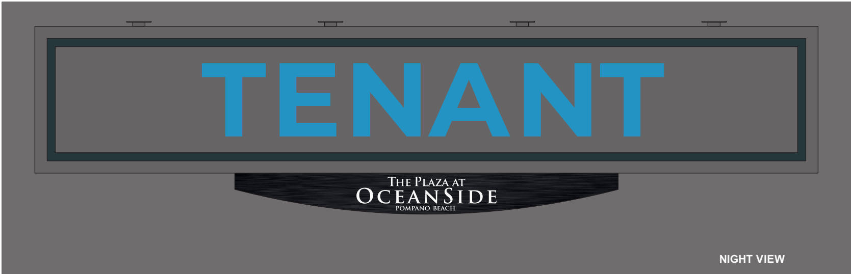
B Hanging Backplate w/ Face Lit Channel Letters, Reverse Lit Channel Border & Illuminated Blade - NIGHT VIEW QTY (1) Scale: 1/2" = 1'-0" Display Sq. Ft.: 54.57
