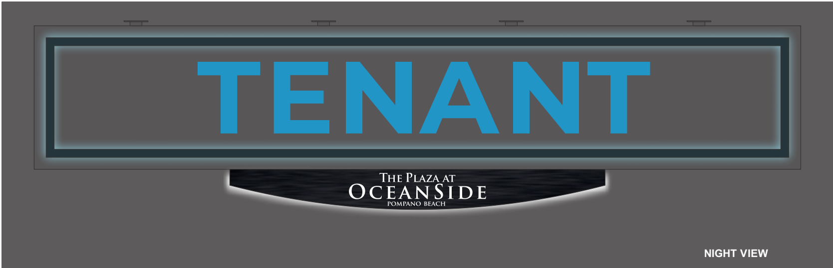
B Hanging Cabinet w/ FaceLit Channel Letters, Reverse Lit Channel Border & Illuminated Blade - NIGHT VIEW QTY (1) Scale: 1/2" = 1'-0" Display Sq. Ft.: 54.57
